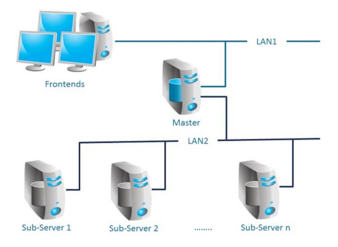
In principle, installation of multiple sub-servers on a multi-processor system is possible. However, when designing the scaling concept, you need to make sure that the scaling effect is not reduced by shared resources. If a shared database instance is used for multiple sub-servers, each sub-server should be assigned individual data files on physically different data carriers.
